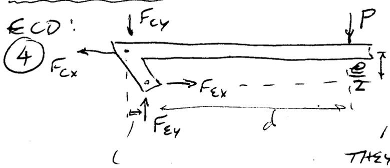
NOTE THAT ONCE THE DIRECTIONS OF  $F_{Cx} + F_{Cy}$  ARE GIVEN IN THE FBD FOR ABC, THEY MUST BE IN THE OPPOSITE DIRECTIONS FOR ECD.
