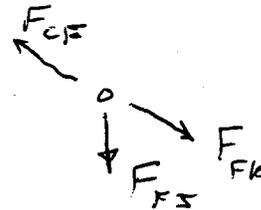
$F_{FS}$  IS THE ONLY FORCE  $\perp$  CFK  $\therefore F_{FS} = 0$
