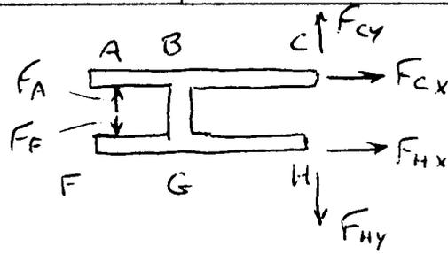
NOTE THAT THE FORCE AT B IS NOT SHOWN SINCE IT IS INTERNAL FOR THIS BODY.
