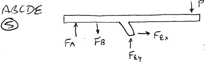
NOTE THAT THE FORCES AT PIN C ARE INTERNAL TO THIS BODY.
