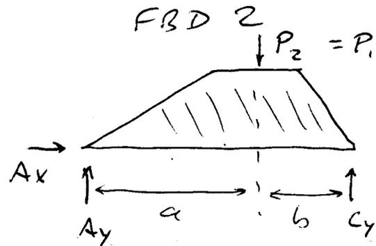
THIS SITUATION OF LOADS OF EQUAL MAGNITUDE ACTING ON A RIGID BODY ALONG THE SAME LINE OF ACTION SATISFIES THE PRINCIPLE OF TRANSMISSIBILITY. WE CAN ALSO SHOW THAT IN BOTH CASES, THE REACTION FORCES ARE THE SAME:
