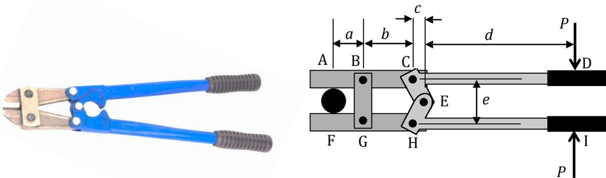
**Problem 4. (20 Points)** The structure shown is loaded by a force  $P$  at the midpoint E of member DF. Because the loading is not at a joint, this structure cannot be treated as a truss.
